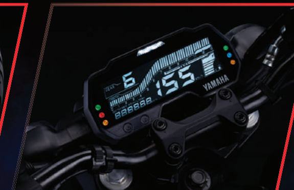
Multi-function Negative LCD Instrument Cluster with Gear Shift Indicator
