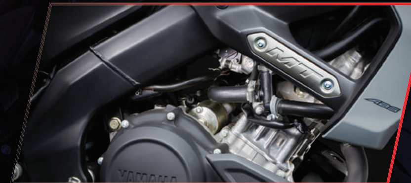
155cc LC4V SOHC Fuel Injection Engine
