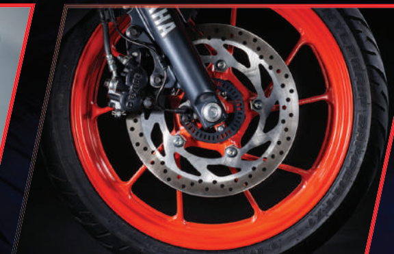
Single Channel ABS with 282 (Fr)/220mm (Rr) Disc Brake
