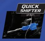
The Quick Shifter\* (up-shift) allows for clutch-less shifting of gears. It increases the comfort of riding the vehicle since it eliminates the need to use the clutch or throttle before and after a gearshift. \*(Standard for R15M & Racing Blue color)
